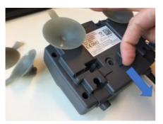
**STEP 3:**Take off the battery compartment cover by pushing it downwards. You can leave the battery installed.
