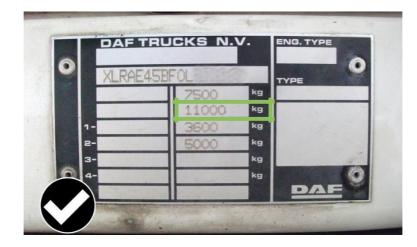
This plate should have the same format throughout Europe. It usually features two columns with weights. The left column represents the national weights, the right column represents the technical weights. You should always register the higher value (in most cases it will be the value in the column on the right). The second row is the value right above the axle weights and always contains the GCWR.
