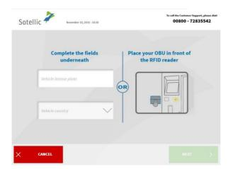
4. You can either place your OBU in front of the RFID reader or fill in your licence plate number and the country of origin of your vehicle. Scanning the OBU in front of the RFID reader is the fastest option.
