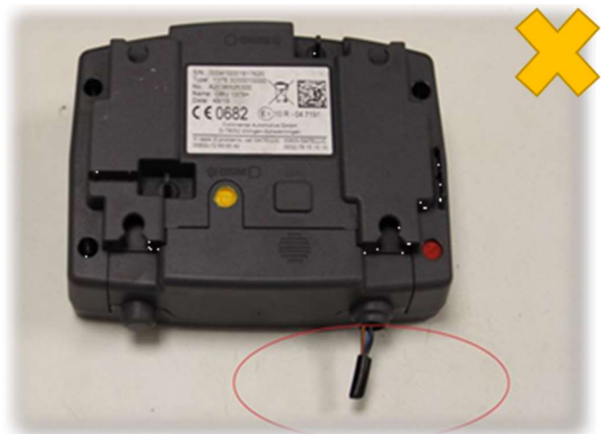
Cut Power Cable
