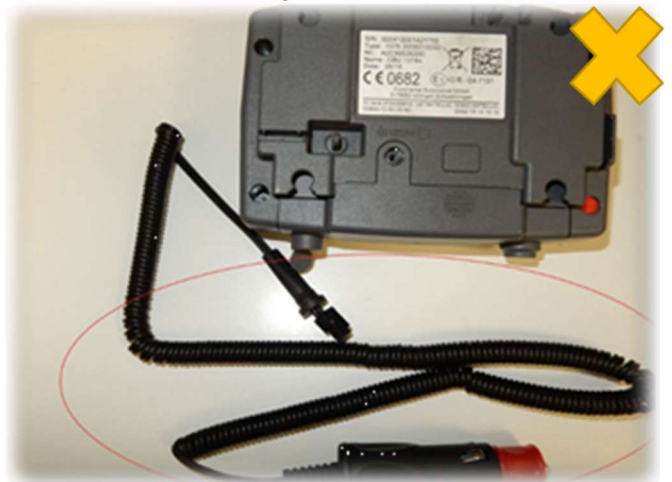
Not Original Power Cable
