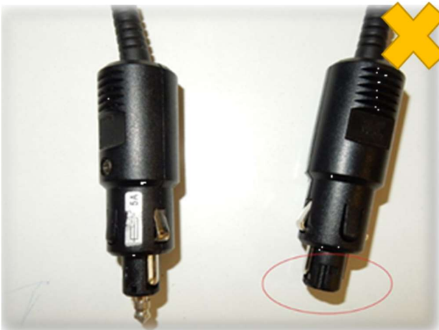
Damaged Power Plug
