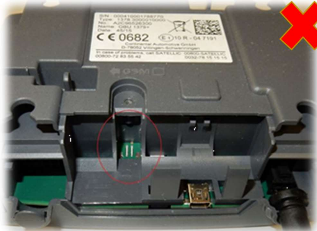
Broken or Missing Connector
