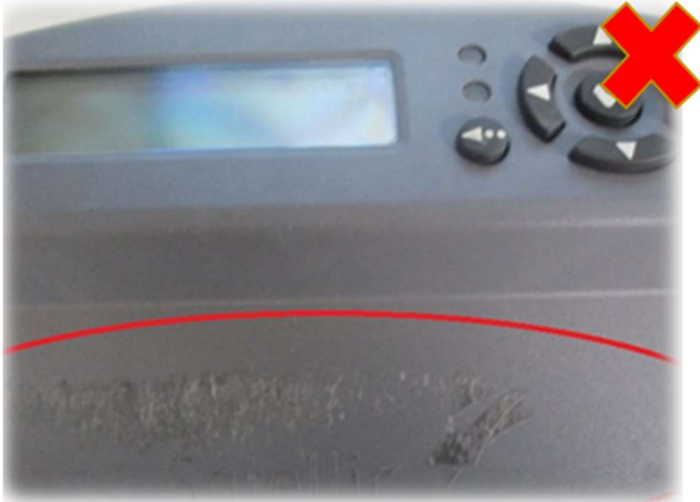
Damages and Scratches
