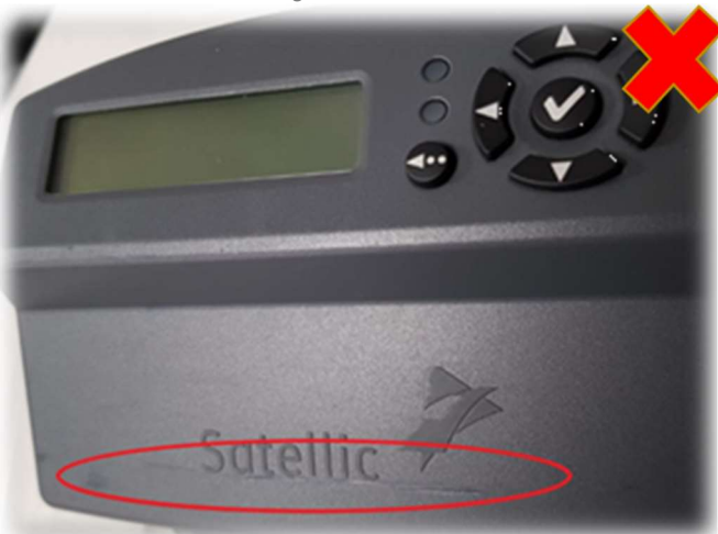
Damages and Scratches
