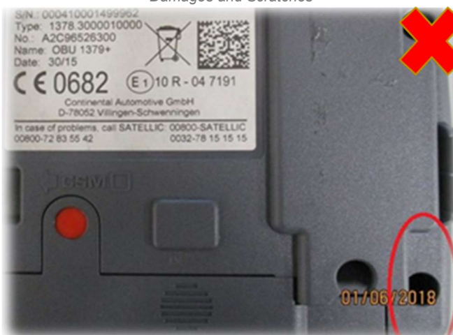
Missing Main Seal
