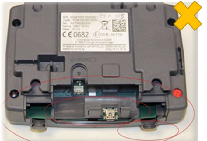
Missing Cable and/or Battery Lid
