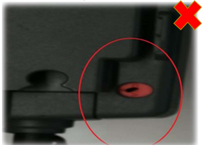
Damages or Broken Main Seal
