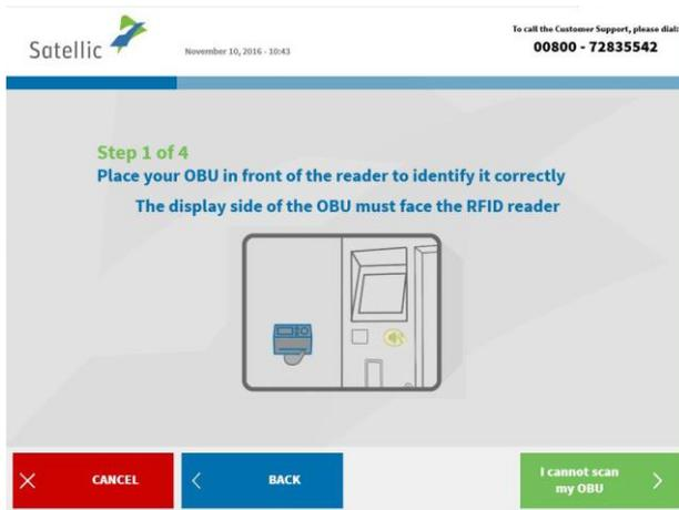
10. Place your OBU in front of the reader to identify it. The OBU has to be turned with the display (front) side facing the RFID reader.
